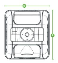
$A > \text{Åpning innkast}^* \mid B > 1180 \text{ mm} \mid C > 1600 \text{ mm} \mid D > 1450 \text{ mm} \mid E > 1600 \text{ mm}$
